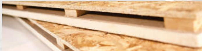
Vented NailBoard® is a rigid roof insulation board composed of a closed cell polyisocyanurate foam core attached with spacers to 7/16" (11 mm) or 5/8" (16 mm) oriented strand board (OSB) on one side and a universal fiber glass reinforced facer on the other.
