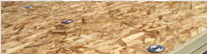
Johns Manville Nailboard® is a rigid roof insulation board composed of a closed cell polyisocyanurate foam core bonded in the foaming process to either 7/16" (11 mm) or 5/8" (16 mm) oriented strand board (OSB) on one side and a universal fiber glass reinforced facer on the other.
